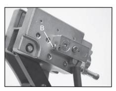
If the lever releases before 60 lbs., using the supplied L-shaped hex wrench, turn the adjustment screw (B) located on the left side of the latch block counter-clockwise to increase the engagement of the brake release latch with the brake lever. Repeat step 1 and adjust until the correct tension is indicated on the calibrator.
