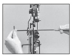
To tighten the braking mechanism, turn the set screw (A) counter clockwise by about 1/8 turn. Re-tighten the allen screw (B) on the back side of the tensioner frame and check for brake tightness. The tensioner should move freely along the track with the brake lever engaged and should hold tension with the brake lever released. If more adjustment is needed, repeat steps above until properly adjusted.
