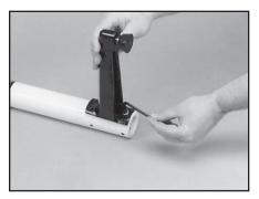
Align the holes in the leg flange with the matching holes in the lower column support post. Secure the leg with one FLAT HEAD cap screw through the upper hole, and one SOCKET HEAD cap screw through the bottom hole. Repeat this procedure for the three remaining legs.
