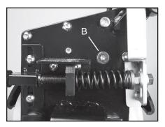
While holding the 5mm brake lever adjustment bolt (A), loosen the hex bolt (B) located on the back side of the tensioner frame with the 4 mm allen wrench.
